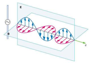
Figure 24.7 A part of the electromagnetic wave sent out from the antenna at one instant in time. The electric and magnetic fields (**E** and **B**) are in phase, and they are perpendicular to one another and the direction of propagation. For clarity, the waves are shown only along one direction, but they propagate out in other directions too.
