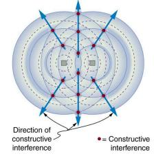
**Figure 24.26** An overhead view of two radio broadcast antennas sending the same signal, and the interference pattern they produce.
