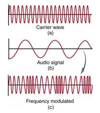
Figure 24.13 Frequency modulation for FM radio. (a) A carrier wave at the station's basic frequency. (b) An audio signal at much lower audible frequencies. (c) The frequency of the carrier is modulated by the audio signal without changing its amplitude.
