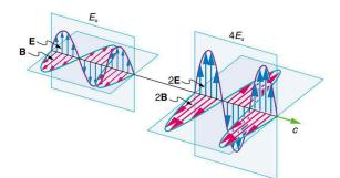
Figure 24.23 Energy carried by a wave is proportional to its amplitude squared. With electromagnetic waves, larger *E*-fields and *B*-fields exert larger forces and can do more work.
