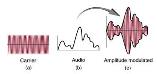
Figure 24.12 Amplitude modulation for AM radio. (a) A carrier wave at the station's basic frequency. (b) An audio signal at much lower audible frequencies. (c) The amplitude of the carrier is modulated by the audio signal without changing its basic frequency.
