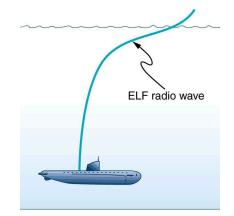
Figure 24.11 Very long wavelength radio waves are needed to reach this submarine, requiring extremely low frequency signals (ELF). Shorter wavelengths do not penetrate to any significant depth.
