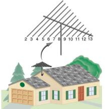
**Figure 24.27** A television reception antenna has cross wires of various lengths to most efficiently receive different wavelengths.
